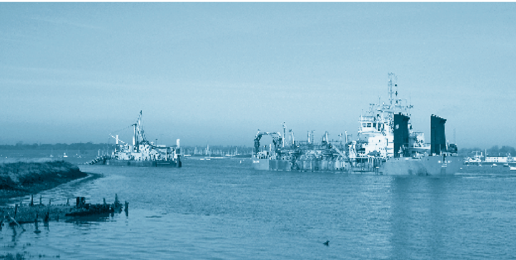
Figure 5. The fine dredged material from maintenance dredging at the Port of Harwich was transported to Wallasea by dredger.
